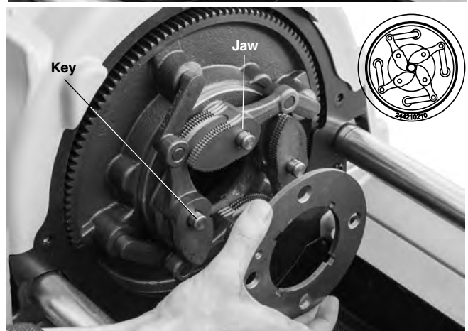
Figure 32 – Changing Auto Chuck Machine Jaws
