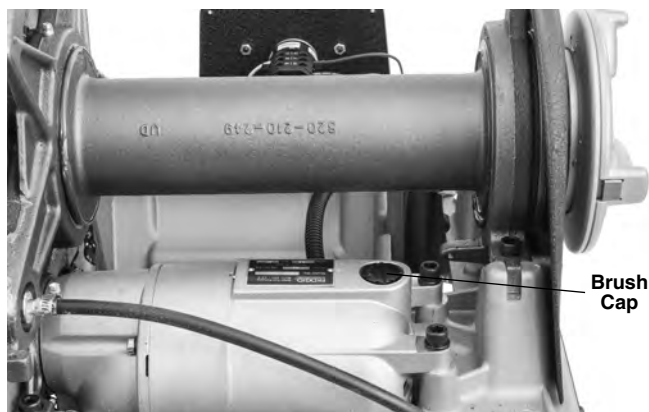
Figure 34 – Removing Motor Cover/Changing Brushes
