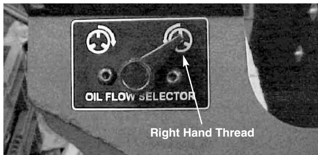
Figure 24 – LH or RH Oil Flow Selector
